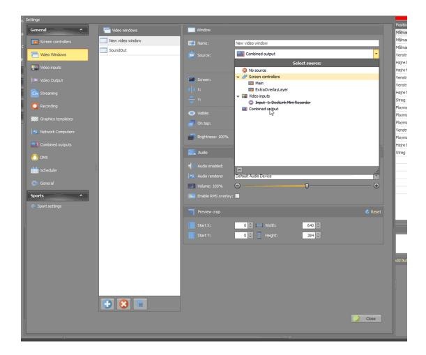
Remove soudn out on that Screen controller and add it on a separate SC. This optimizes the sound and mimizes issues of sound lagging.
